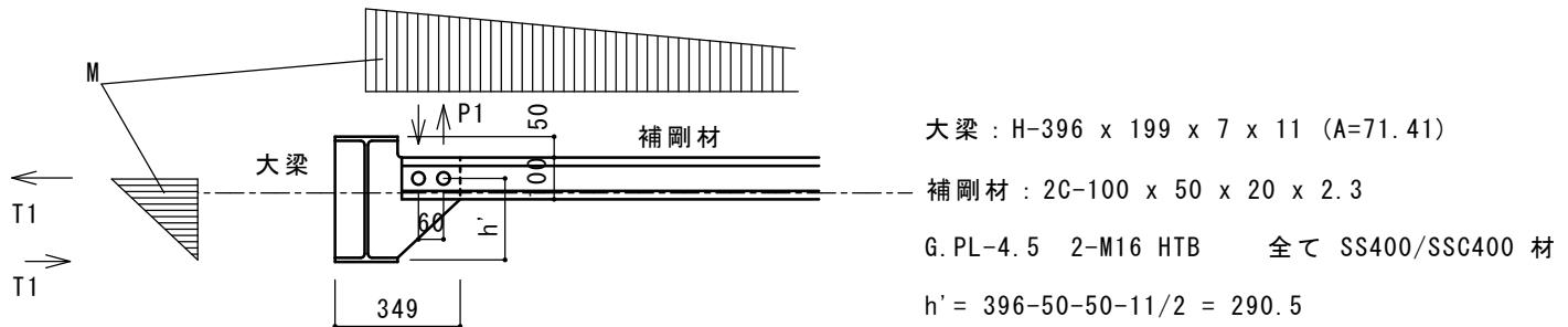
$$T_1 = 71.41/2 \times 23.5 \times 1.1 \times 0.02 = 18.5 \text{ kN}$$
